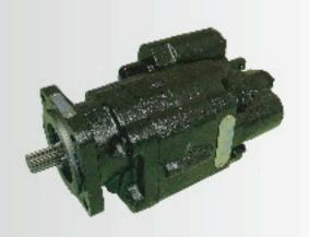
The C102D direct mount gear pump does not require a drive line thus making it safer and more dependable. This pump has an S.A.E. "B" 4-bolt flange and is used for heavy duty hoists. 25 GPM @ 1200 RPM
