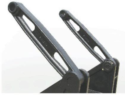
Shown is the heavy duty cast lift arms. These arms easily attach directly to the body using 4140 grade, 1 1/2" hinge pins which are bolted in place with grade 8 bolts.
